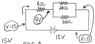
so the battery supplies  $I = \frac{V}{R} = \frac{15V}{20\Omega} = 0.75 \text{ A}$
