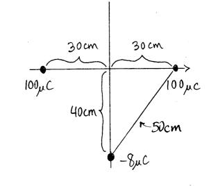
In this problem the 100mc charges produce a field that the -8mc charge moves in. We can find PE using PE=gV where V is the electric potential 100mc
