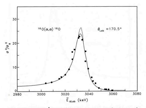
Fig. 2. Measured  $^4$ He-O laboratory cross sections near the strong "3045" keV resonance are compared with values (solid line) calculated using Cameron's procedures [3] and our resonance parameters listed in table 3, including the effect of target thickness. The dashed curve is the result of the calculation for infinitesimal target thickness. The data points shown were taken with the thin (6 keV) target. We obtain the resonance energy of  $(3034\pm4)$  keV.
