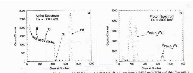
Fig. 6. (a) Energy spectrum of backscattered (170.5° lab angle) 3000 keV <sup>4</sup>He <sup>+</sup> ions from a Pd(32 nm)/B(96 nm) thin film with a Si(4 nm) cap on a Si substrate. The collected charge was 50 μC. (b) Energy spectrum of protons (135° lab angle) taken simultaneously with the alpha spectrum of fig. 6a.
