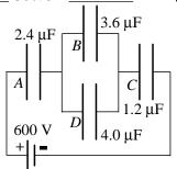
$$\begin{split} &C' = C_{_B} + C_{_D} = 3.6 \,\mu\text{F} + 4.0 \,\mu\text{F} = 7.6 \,\mu\text{F} \\ &\frac{1}{C} = \frac{1}{C_{_A}} + \frac{1}{C'} + \frac{1}{C_{_C}} = \frac{1}{2.4 \,\mu\text{F}} + \frac{1}{7.6 \,\mu\text{F}} + \frac{1}{4.2 \,\mu\text{F}} = \frac{1}{0.72 \,\mu\text{F}} \end{split}$$
