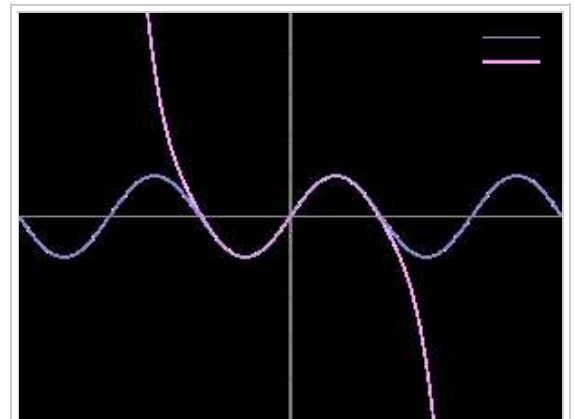
The sine function (blue) is closely approximated by its Taylor polynomial of degree 7 (pink) for a full cycle centered on the origin.
