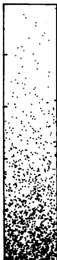
Figure 2-20 Equilibrium height distribution of particles in a gravitational field. The distribution is the same as that given by the law of atmospheres, n(z) = n_0 e^{-mgz/kT} . (This computer-generated plot courtesy of Paul Doherty, Oakland University.)
