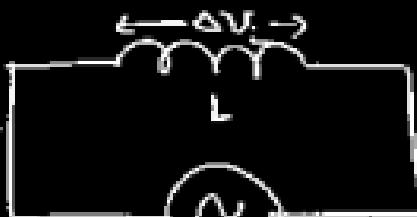
$$\Delta V = \Delta V_{\max} \sin \omega t$$
