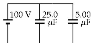
(a)  $C_p = C_1 + C_2 = 25.0 \mu\text{F} + 5.00 \mu\text{F} = 30.0 \mu\text{F}$
