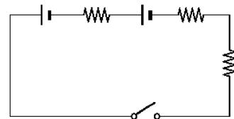
$$(a) \quad R_{\text{lamp}} = R - r_{\text{batteries}} = 5.00 \Omega - 0.408 \Omega = \boxed{4.59 \Omega}$$
