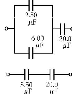
$$Q = C\Delta V = (6.00 \mu\text{F})(10.53 \text{ V}) = 63.2 \mu\text{C}$$
