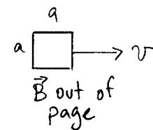
$\vec{v} = v\hat{x}$  through a field that increases linearly with  $x$ ,  $\vec{B} = (B_0 + \alpha x)\hat{z}$ .
